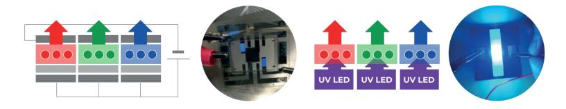
**PureBlue.dots** applied in electroluminescent device as optically active layer for new technology of displays.
